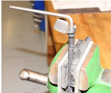
Unscrew foot bolt, remove foot. Installation is the reverse of removal.
